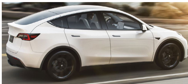
On the newly released 2020 Tesla Model Y, the entire rear of the car is on the same line, providing no protection for the rear liftgate in the event of a rear collision.
